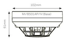
The optical-thermal detector conforms to EN54-7, a 58°C fixed temperature and rate of rise thermal assistance conforming to EN54-5. The thermal detection function combines thermistor technology with a software corrected linear temperature response. In areas where the normal daytime activities may potentially create unwanted alarms, the detector can be programmed to operate in a "heat only" mode, automatically reverting to full photo-thermal operation during unoccupied periods.
